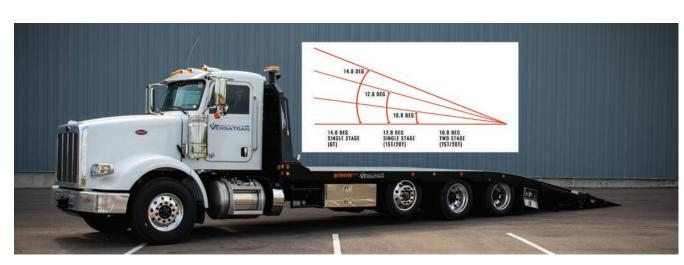
Patented Bed Design - The Retriever's curved deck creates the lowest loading angle of any similar product. 12.8 degree for single stage ramp on a 15 or 20T. 10.8 degree for two stage ramp on a 15 or 20T. 14.0 degree for single stage ramp on a 6T.
