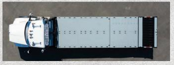
Secure equipment using the available 140 chain slot tie-down points strategically located at the perimeters and center of the Versatran 20T Retriever bed. This allows securement for side-by-side transportation of equipment. Key slot tie-down points are a standard 20T offering.
