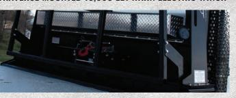
The traverse mounted 15,000 lb. Warn electric winch allows you to load inoperable equipment up the ramp on its own. The Warn winch is a standard 20T feature. Also shown, optional winch guard for added protection when loading and unloading equipment.
