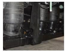
Proven Air System - Industry leading Firestone® air bags are engineered to operate the Retriever deck and ramp systems.
