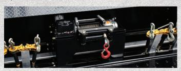
The 15,000 lb. Warn electric winch provides the capability to load non-powered equipment onto the deck. The Warn winch is a standard 6T feature.
