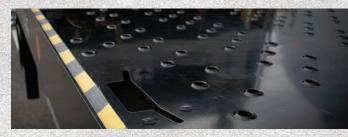
Slip-resistant, debossed tread deck provides maximum traction to equipment driving on the ramp. The 6T Retriever also has 68 total key slot tie-down points.
