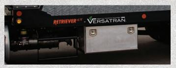
Large aluminum toolbox, 18" x 18" x 36", with single door mounted on the drivers side. Also pictured is the deck access step. Both features are standard 6T offerings.
