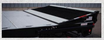
The air-operated Retriever deck and ramp system are the envy of the industry. Depending on equipment load size, unit can travel with the ramp flat on deck or locked in the vertical position for maximum capacity.
