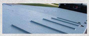
Slip-resistant, epoxy-coated deck provides maximum traction to equipment driving on the ramp. Also shown, optional deck cleats for steel track equipment. Other options include expanded metal for additional traction.
