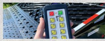
Wireless remote allows operators to operate the 6T Retriever deck from a safe location or even the equipment seat. The wireless remote is a standard 6T feature.
