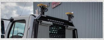
Stay safe on the worksite with the 15T Retriever's array of lighting offerings. Pictured are the 15T Retriever's standard LED mini light bars and upper and lower work lights provided as standard features.
