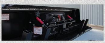
The traverse mounted 15,000 lb. Warn electric winch allows you to load inoperable equipment up the ramp on its own. The Warn winch is a standard 15T feature.
